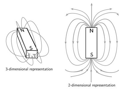
In areas where the magnetic field is strong, the field lines are closer together. Where the field is weaker, the field lines are drawn further apart. The strength of a magnetic field is referred to as the **magnetic flux**
