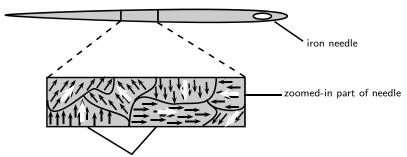
in each domain the electron magnetic fields (black arrows) are pointing in the same direction, causing a net magnetic field (big white arrows) in each domain
